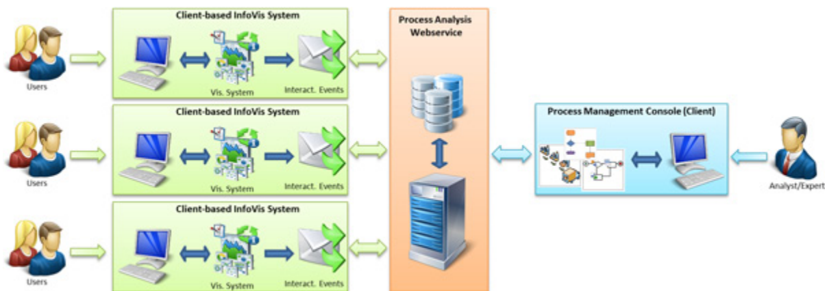
Figure 4. An overview of the entire Process Analysis Architecture. In general, multiple instantiations of the visualization client are used at the same time. All events on the system are sent to the process analysis web-service, which generates a process model semi-automatically. Based on the process model the user gets actively supported during his further system use.
