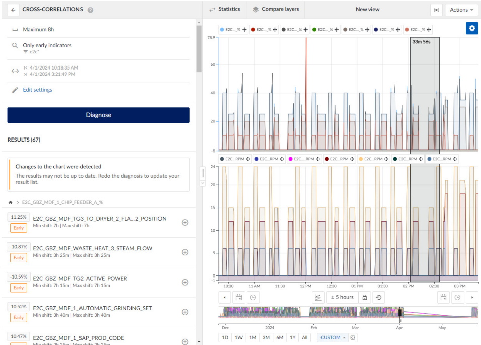
Fig. 8: A cross-correlation analysis performed on early indicators to identify potential root causes
